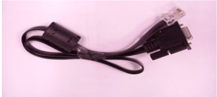
Flat Cable (RJ-45 to DB-9F flat cable onnector)
